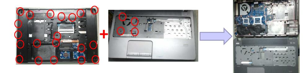
Loose L-case to U-case screws on bottom side & U-case to L-case screw on top side, and take off U-case from system.
